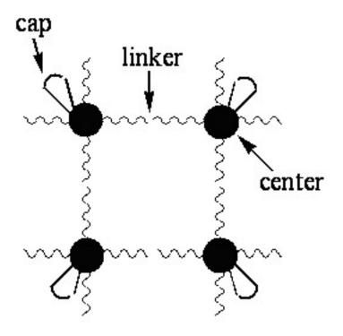
The initial phase in development of such a grid material is the connection of two Mo centers that contain "cap" ligands.
