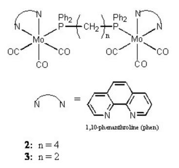
In reactions of  $Mo(CO)_4$ (phen) and diphosphines using 2:1 or 1:1 mole ratios, we have prepared the novel bridged dppb and dppe complexes **2** and **3**, respectively. UV-vis, IR, and NMR (<sup>1</sup>H and <sup>31</sup>P) spectroscopy confirm the stoichiometry and the nature of diphosphine coordination in these complexes. Work on expanding this type of structure to a "square" as well as utilizing diisocyanides as bridging ligands is underway.
